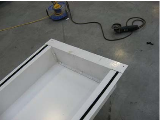
9. Place expandable foam tape around plenum edge.
